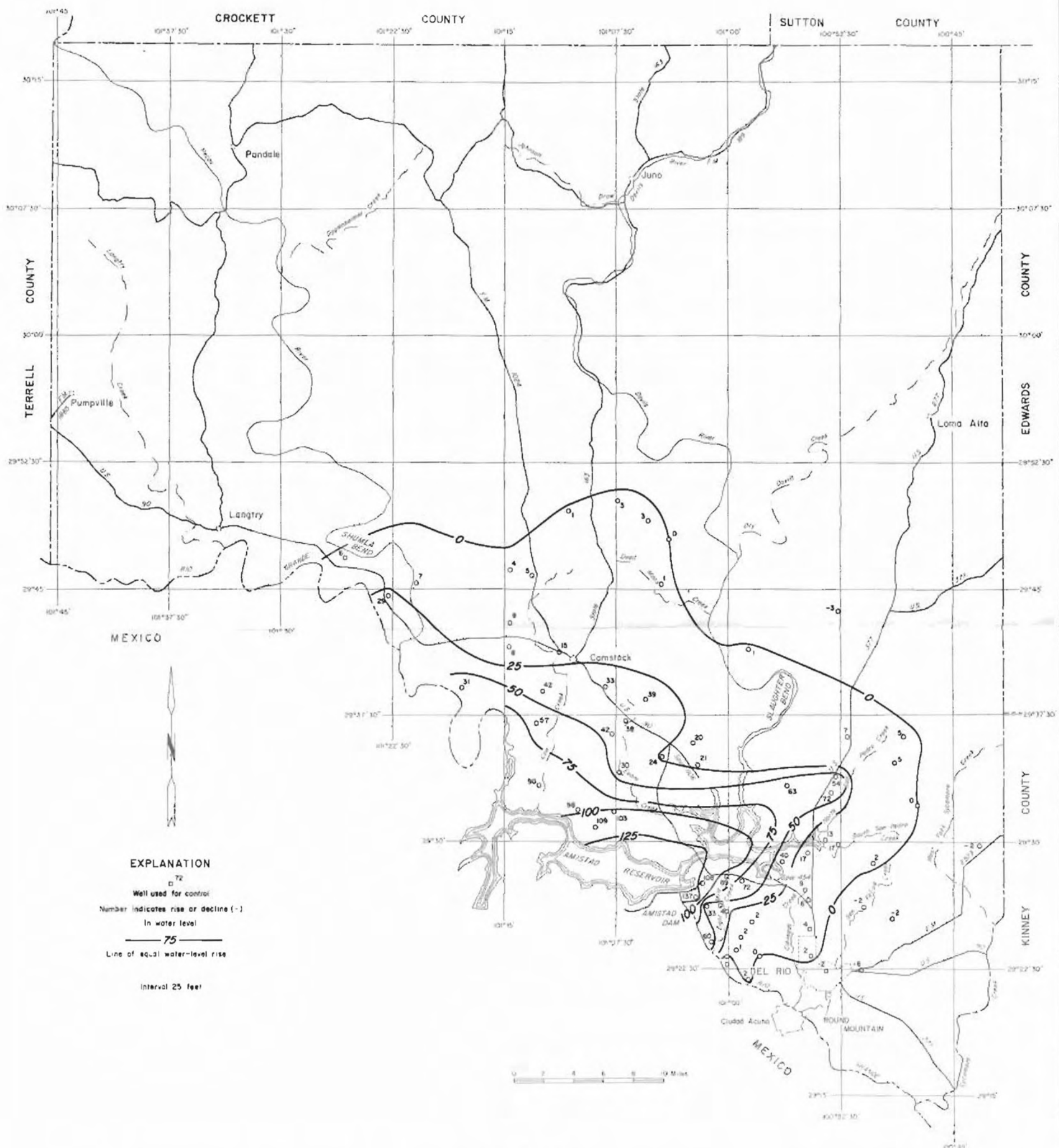
Figure 15 Approximate Net Changes of Water Levels in Wells Tapping the Edwards and Associated Limestones Due to Water Impoundment in Amistad Reservoir From July 1968 to July 1969
